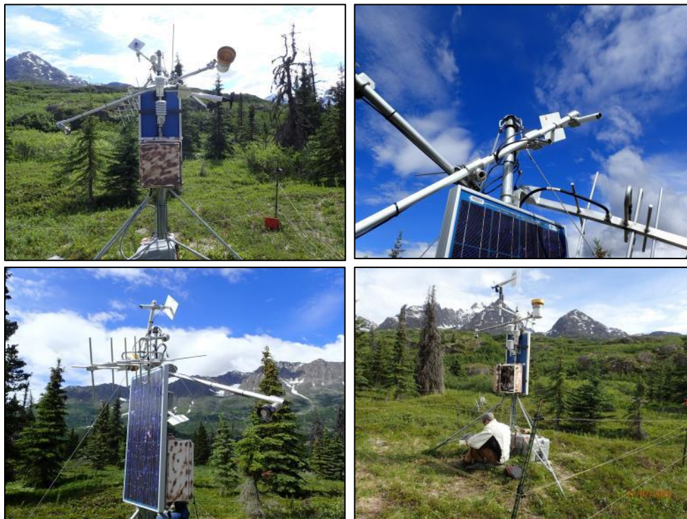
Figure 14. Tebay station June 28, 2016. The crossarms had been sheared off by snow loading. The guy wires were removed and all sensors were re-leveled during the field visit.
