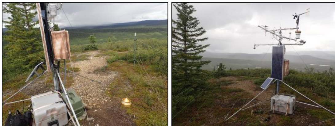
Figure 17. Upper Charley station July 6, 2016. The lid of the tipping bucket was on the ground upon arrival at the site (left).
