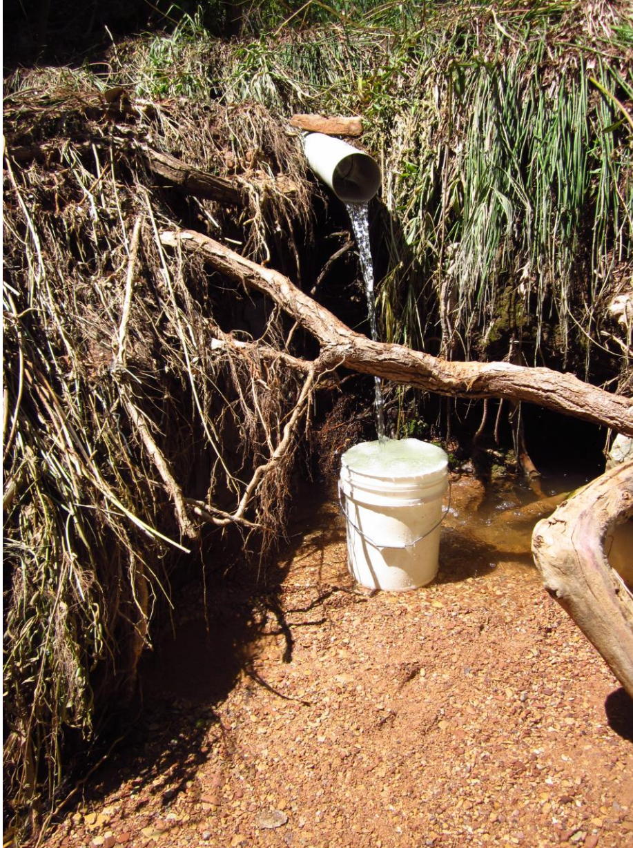
Figure 2. Example volumetric measurement using a pipe and bucket.
