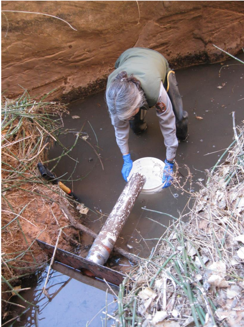
Figure 1. Example volumetric measurement using a temporary weir and bucket.
