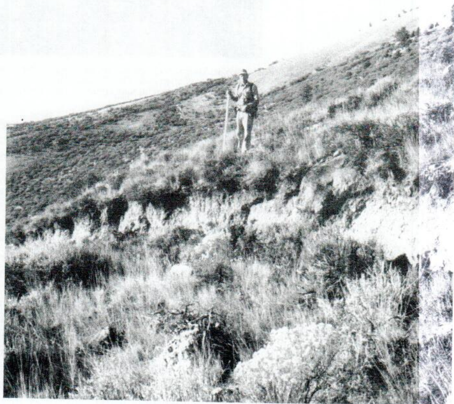
FIG. 13. Largest scarp on the northern section of surface faults (see Plate 2). Net throw is 1.0 m, and scarp height is 1.2 m. Pattern of ground breakage on this section is generally simple compared to the patterns on the other sections. Photograph by W. E. Scott, 29 October 1983.
