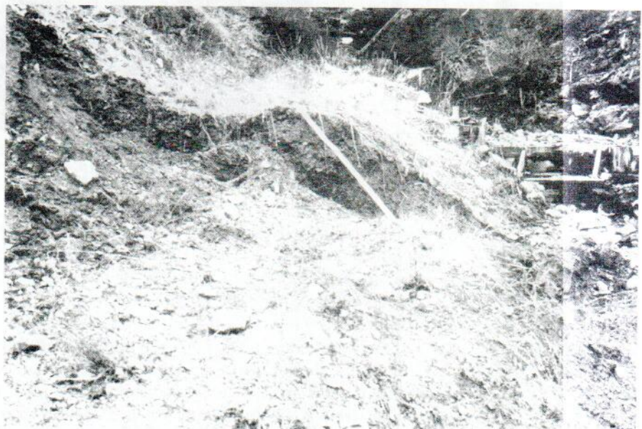
FIG. 7. Faulted jeep trail near western base of Dickey Peak at northwest end of southern section (see Plate 2). Net throw is 0.90 m, and sinistral slip is 0.65 m. Stadia rod shows separation of two previously connected points. Rod is 1.5 m long. Photograph by W. E. Scott, 2 November 1983.
