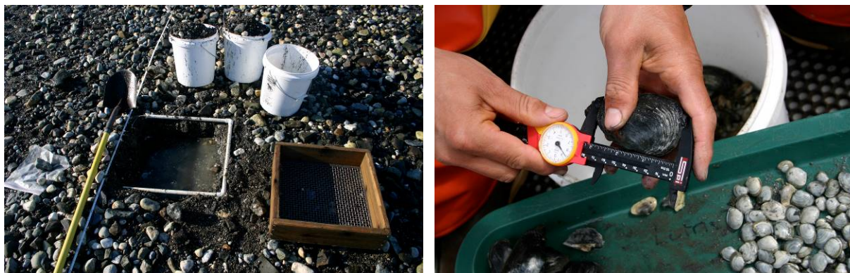
Figure 3. An excavated quadrat is ready for sieving. Left (A) – Image of a quadrat and sampled area, 10 mm mesh sieve, 3-5 gallon buckets for containing sediment, shovel, transect tape, and a labelled clam collection bag. Note that the water is to the left of the transect tape, such that the lower left corner of the quadrat lies on the meter mark. Right (B) – An observer carefully measures a large Mya truncata with other clams sorted in the background. All bivalves are identified, counted, and measured by quadrat.
