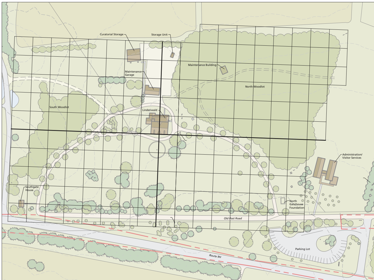
Figure 3.35. Diagram illustrating a sample geophysics collection grid established from fixed base points (east facade and centerline of mansion). Establishment of a grid system will allow data collected through multiple projects and investigations to be linked for comprehensive analysis, 2016 (OCLP).
