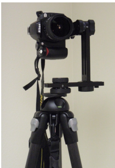
Figure 4. Nikon D40x with Nikkor 16mm 2.8D fisheye lens mounted on a Nodal Ninja panoramic head.
