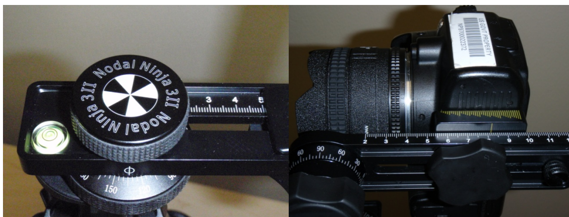
Figure 5. The correct positions for a Nikon D40x and 16 mm lens on the Nodal Ninja 3 Mk II.
