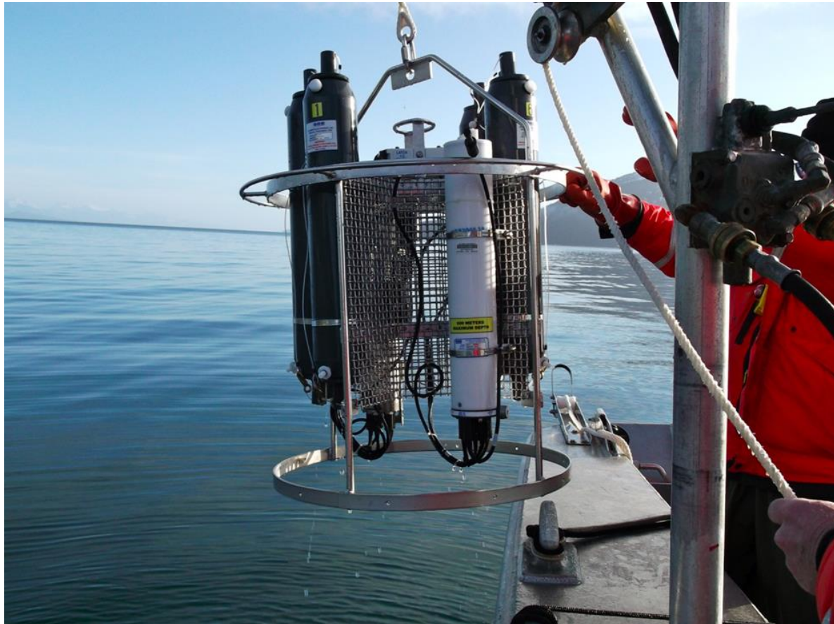
Figure 2. The CTD integrated with the rosette bottle sampler being recovered (bottles closed, containing water samples from known discrete depths) following a cast.
