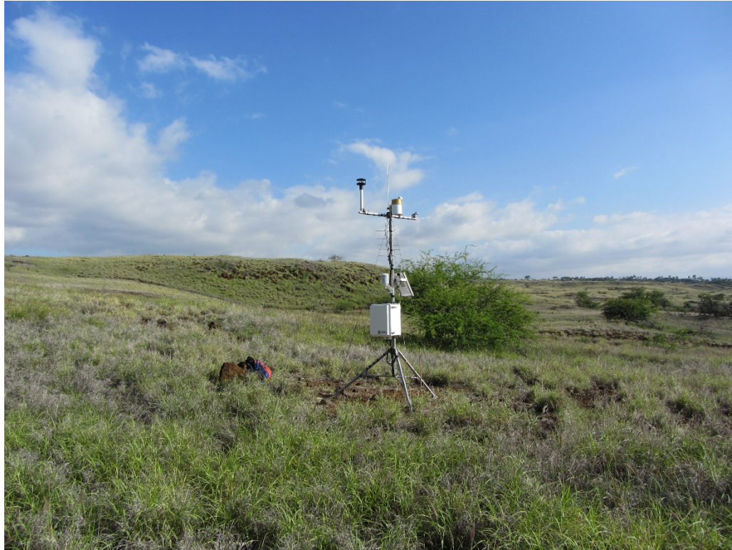
Figure 1 – Replacement climate station installed at Pu'ukoholā Heiau NHP in January 2015.
