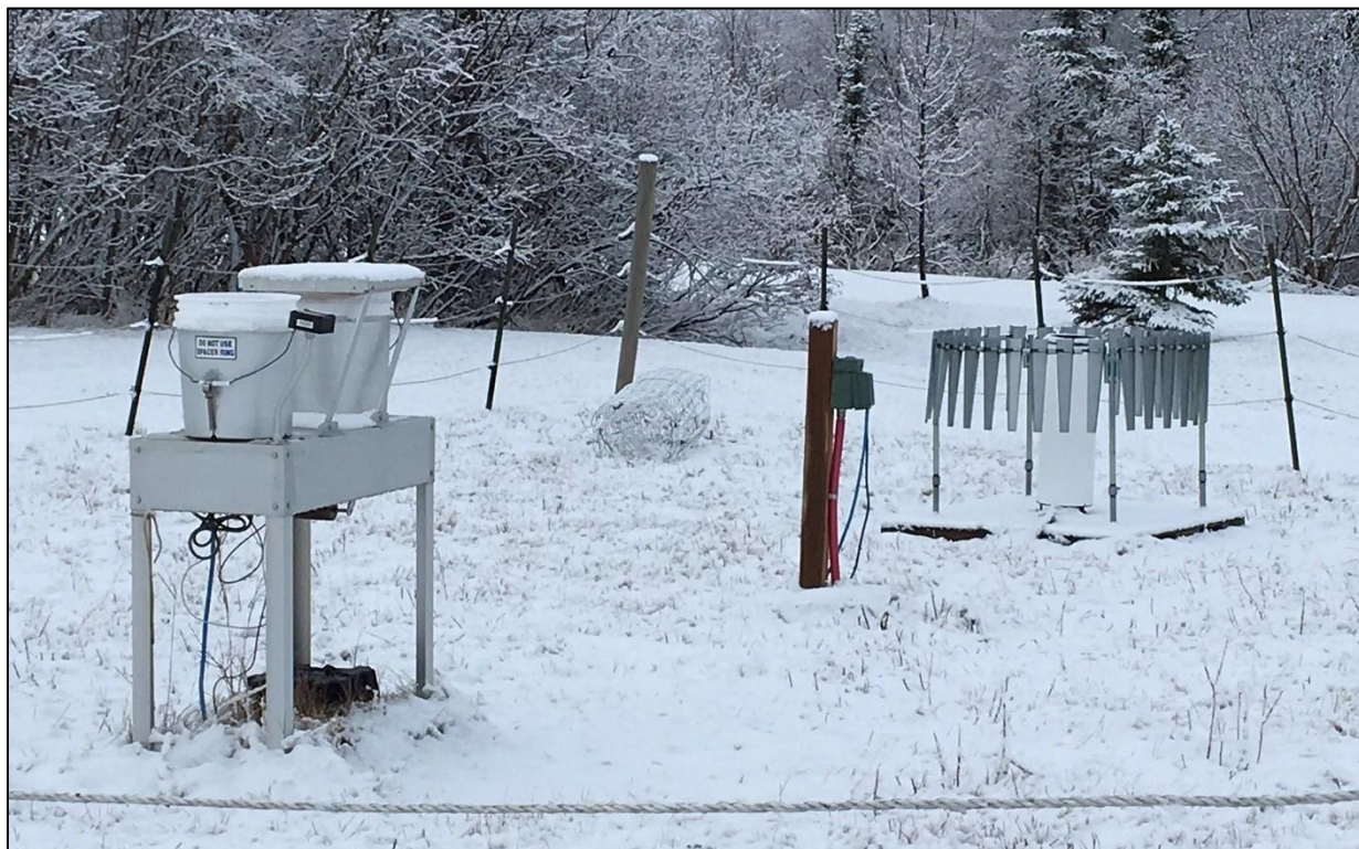
Figure 3. The precipitation collector (left) and raingage (right) used to monitor wet deposition at AK97.
