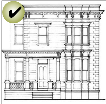
Preferred Approach, when historic documentation is available: Italianate style house with a replacement porch designed similar to that seen historically.
