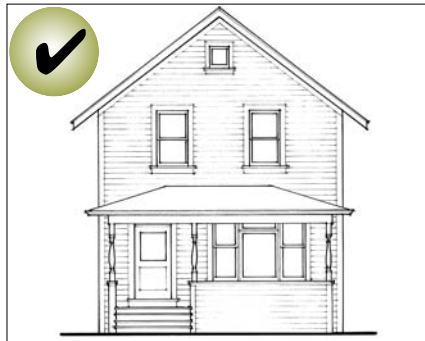
Preferred Approach, when historic documentation is available: A folk or vernacular style house with a replacement porch designed similar to that seen historically.
