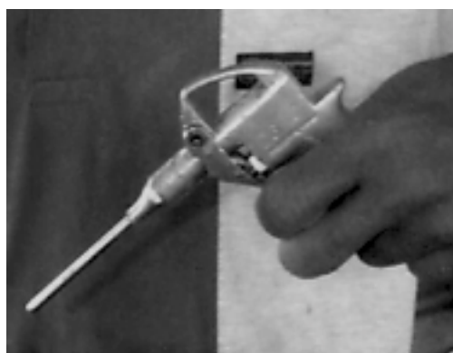
Figure 58. Recommended oxygen nozzle shape and size. (Larry Sharron).
