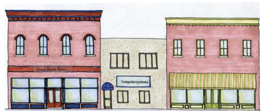
Example of an incompatible infill (center structure) utilizing inappropriate materials and color that do not match the red brick of the neighboring commercial structures. This infill also does not match the pattern (repetitive elements of the windows and storefronts) or massing (height) of the adjacent buildings.
