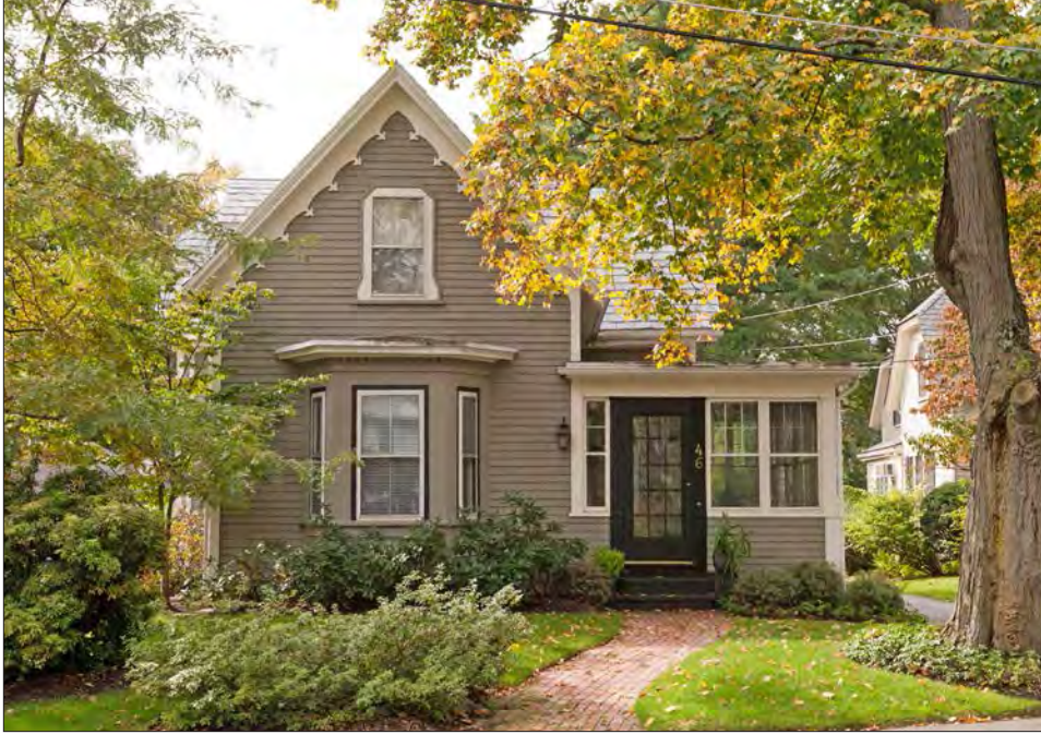
The majority of Gothic-Revival structures in Newton - such as this house in Auburndale - are in the style known as Carpenter Gothic, in which Gothic details such as decorated vergeboards and finials are constructed in wood (note that the porch enclosure in this example is a later alteration).
