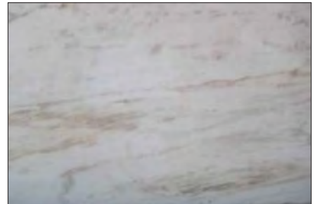
Marble - Typically fine grained and able to be highly polished; it has a wide range of colors and patterns; used for steps and stoops, statuary and fine masonry.
