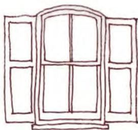
The 2-panel shutters do not fit the arched opening of the window
