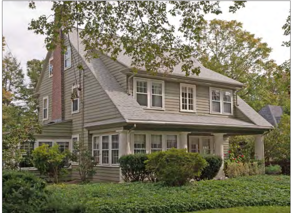
This bungalow in Auburndale features a gable roof, wide and shallow shed-roof dormer, and a full-width, recessed porch supported by columns extending to grade
