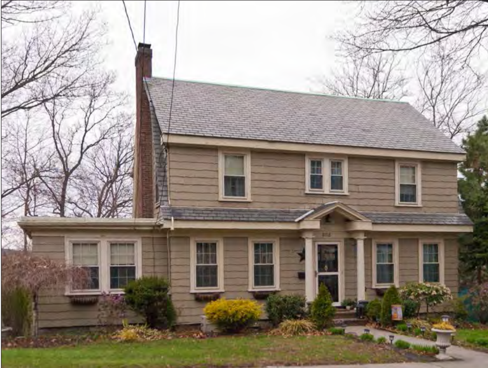
This Dutch-Colonial Revival house in Auburndale features a side-gambrel roof (with full-width dormer) and a prominent central front entry door.
