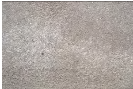
Granite - A hard rock, consisting of small, yet visible, grains of minerals, which can be highly polished or textured; used for walls, piers, columns and street curbs; commonly in gray, black and pink.
