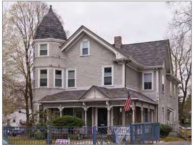
Often, additions or alterations to historic buildings can make it difficult to assign a single style. This Italianate house at 410 Newtonville Avenue - which has a preservation restriction held by the City - has a turret with Queen-Anne detailing that was added as a later alteration.
