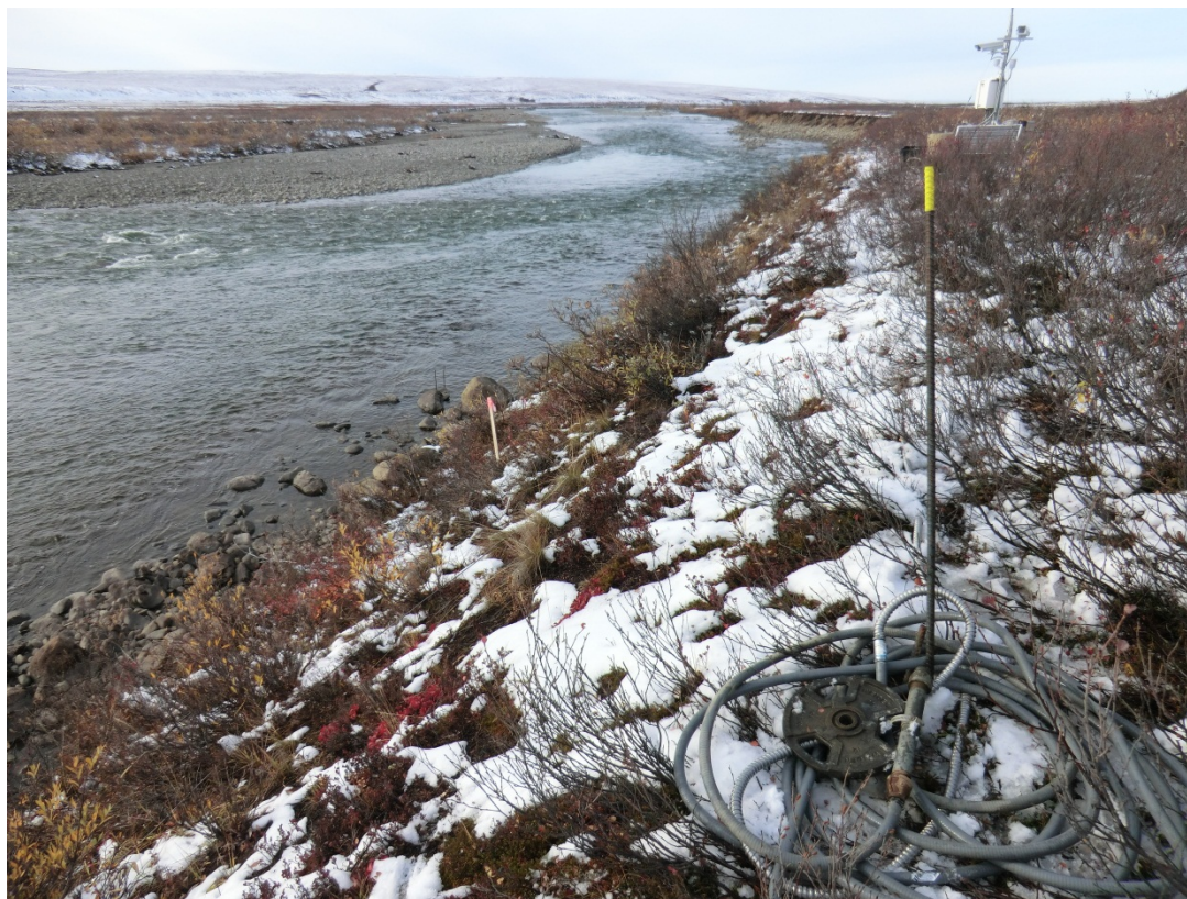
Figure 2. Itkillik River Station. Rebar is used for temporary benchmarks and to secure sensors.
