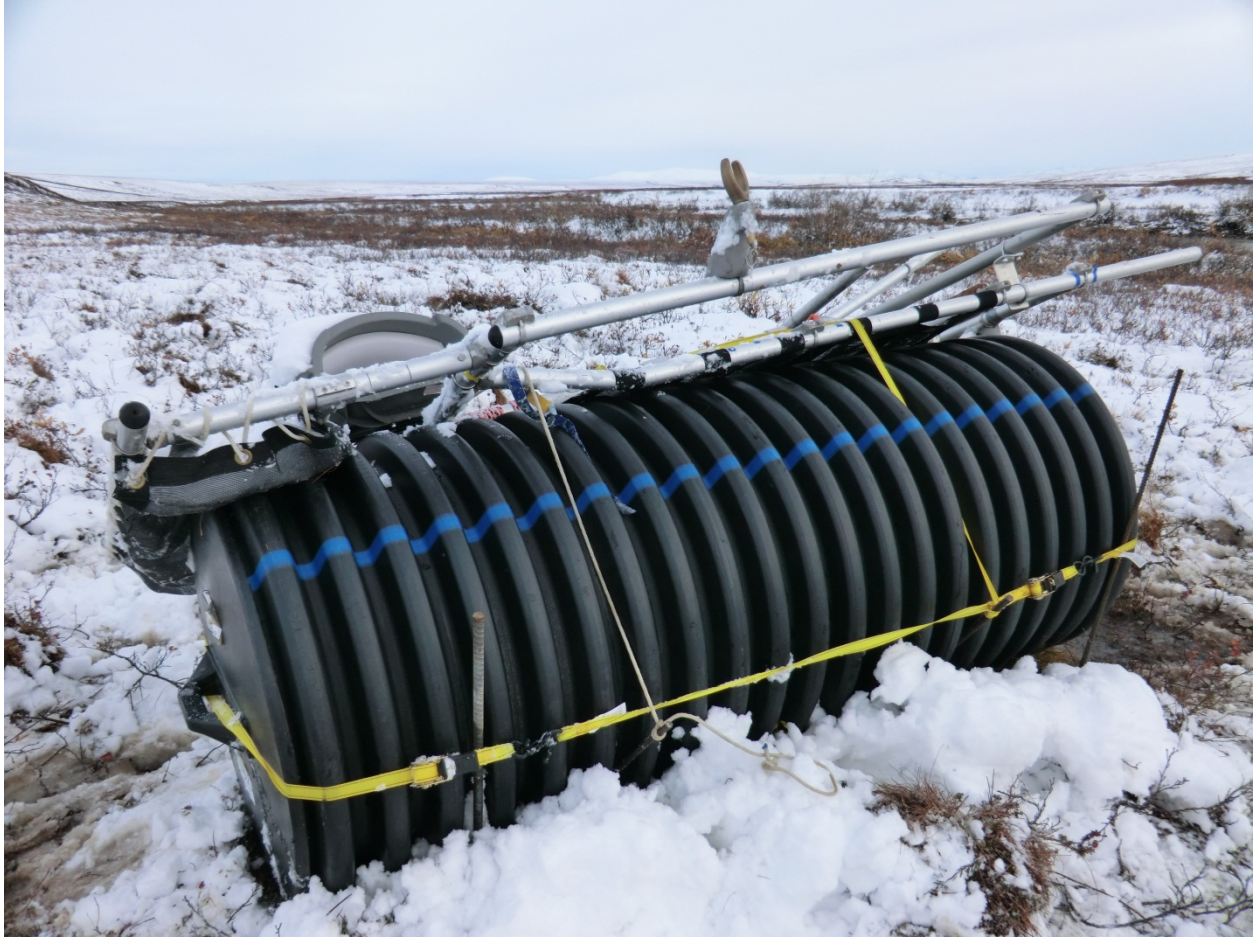
Figure 3. Storage unit at the river for keeping boat, motor, and safety equipment protected from weather and animals. The storage unit could be camouflaged, hidden out of site of the river, and/or placed in a location in the forest. This example shows a cataraft frame at the river but it is proposed that a zodiac would be used at the Kobuk station. The zodiac would be stored inside a container for safe keeping.
