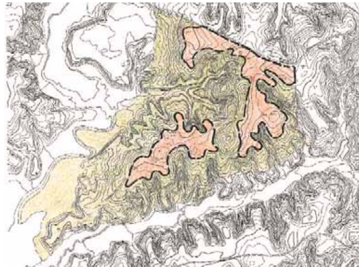
The site's hydrology, topography, and soils limit development to only 35 of the site's 196 acres.
