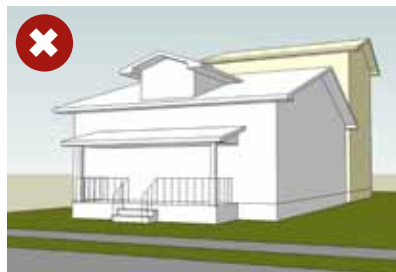
Two-and-a-half story addition with connector Addition overwhelms the original house, and con- nector is not sufficient to separate.
