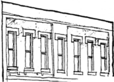
Existing building with missing cornice.
