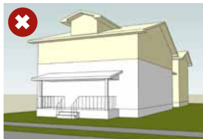
Two story roof-top addition Addition removes origi- nal roof and removes the ability to perceive the historic significance of the structure.
