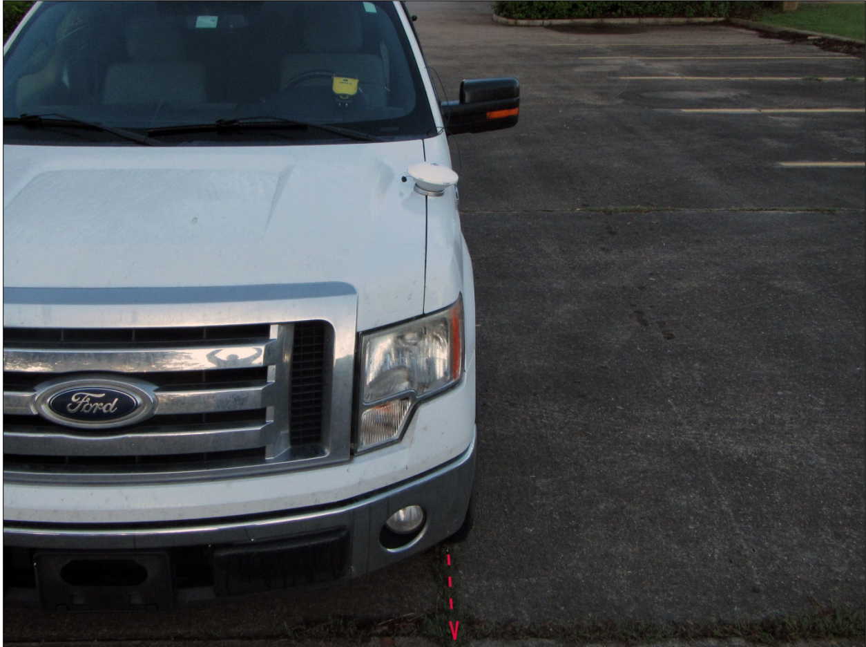
Figure 15. Data logger antenna mounted on a 4x4 vehicle. Red/dashed arrow indicates path of vehicle (simulated swash line).
