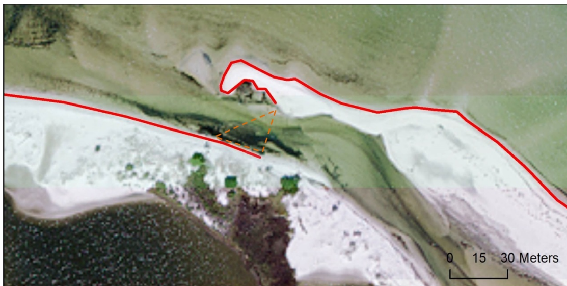
Figure 22. Mapping shoreline inlets. The solid red line represents the surveyed shoreline. The orange dotted triangle indicates a line that is perpendicular to the general orientation of the inlet. The surveyor should capture approximately 30 meters of the inlet margins at its opening.
