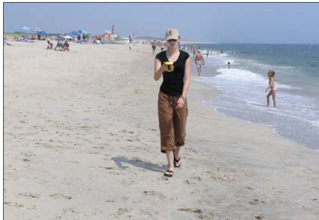
Figure 20. Conducting the survey and holding the GPS/GNSS data logger. The operator walks along the wet/dry line on the beach face to capture the position of the neap high-tide swash line. Figure and caption from Psuty et al. (2010).
