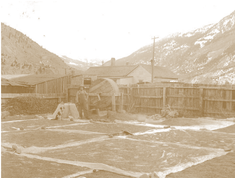
Seed extractor or cone tumbler. Open cones are placed into the extractor; then the drum is turned over, shaking the remaining seed out of the cones. There may be paddles inside the drum to knock the cones around more. The seed being smaller in size than cones will fall to the bottom of the drum. Most seed extractors should have a screen on the outside of the drum which allows the seed to fall through and out while keeping the cones and larger debris in. On the photographs, the detail of the screens and fill/empty hatches is not readily apparent. Bushel bags are the common unit of measure for cones. Contractors were paid by the bushel for collected cones. Extracted seed is usually measured by the pound. Bags on the right appear to be filled with clean seed, which is the end product of the process.
