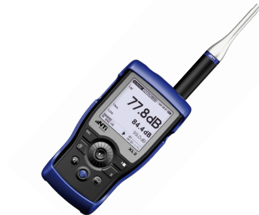
Figure 12: NTi XL2 Audio and Acoustic Analyzer
