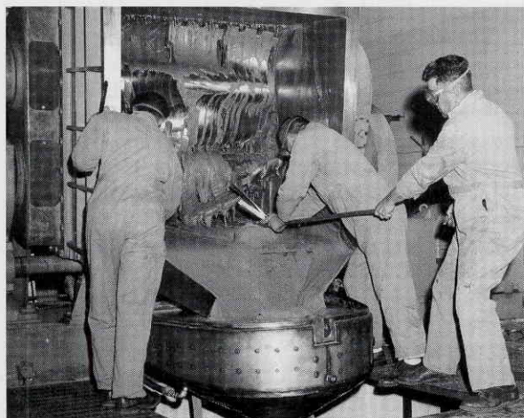
Thiokol Chemical Corporation technicians cleaning a mix of solid propellant out of a 300-gallon mixer. The propellant was used in Thiokol's first-stage engine for Minuteman missiles (n.d.).
