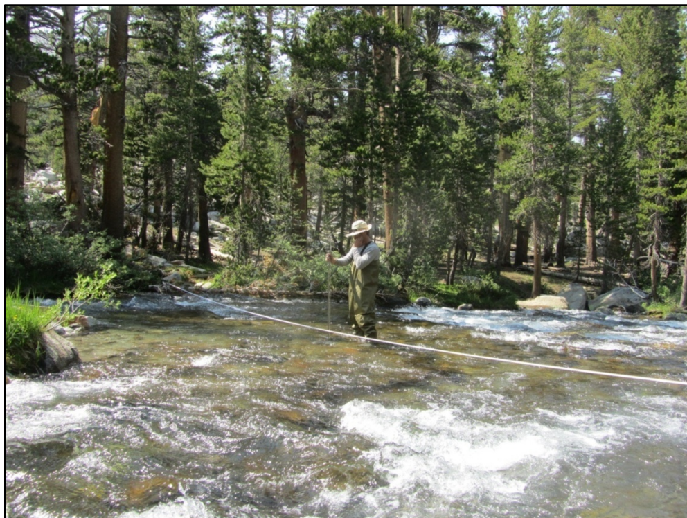
Figure 1.3. A technician performing a discharge measurement approximately 75 meters upstream of the Lyell Fork streamgage.
