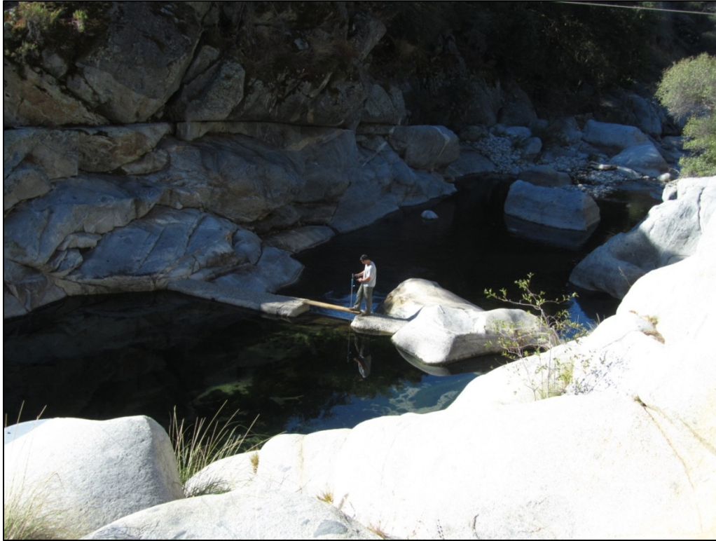
Figure 1.10. SCE hydrographer collecting a low flow discharge measurement at the concrete gage control at the Middle Fork Kaweah streamgage.
