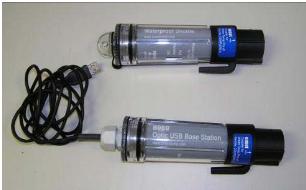
Figure 3.4. HOBOWare shuttle and coupler. The coupler is the black portion on the right side of the photo.
