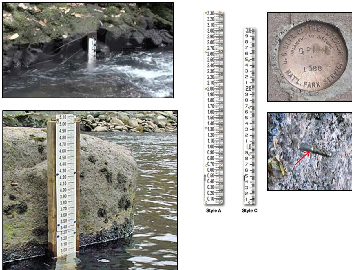
Figure 2. Examples of staff plates installed flush against rock, Style C versus Style A, and examples of a NPS Benchmark versus rock bolt.
