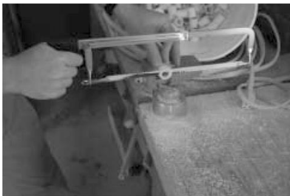
Figure A.1. First cut on PVC.
