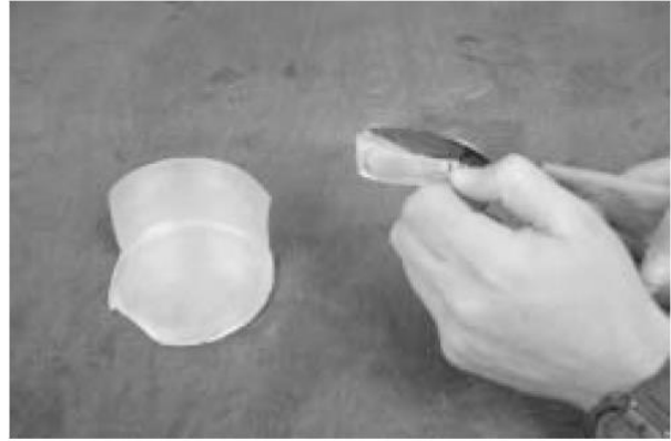
Figure A.5. Cutting shovels with tin snips.
