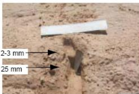
Figure 5. Excavate trench for subsurface sample.
