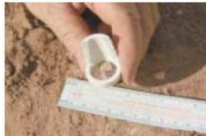
Figure 3. Ensure correct sample size.
