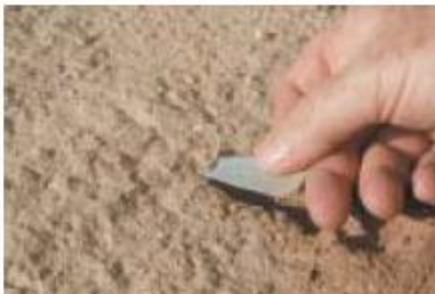
Figure 2. Collect surface sample.
