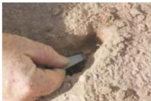
Figure 6. Collect subsurface sample.
