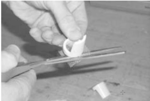
Figure A.4. Cutting out baskets from screen.
