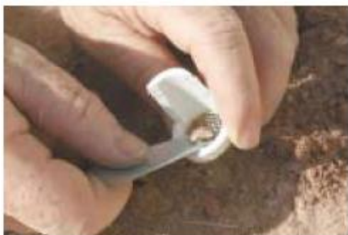
Figure 4. Place sample in sieve.
