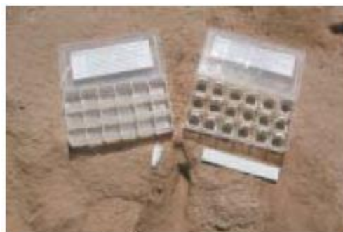
Figure 7. Complete soil stability kit with water and samples.
