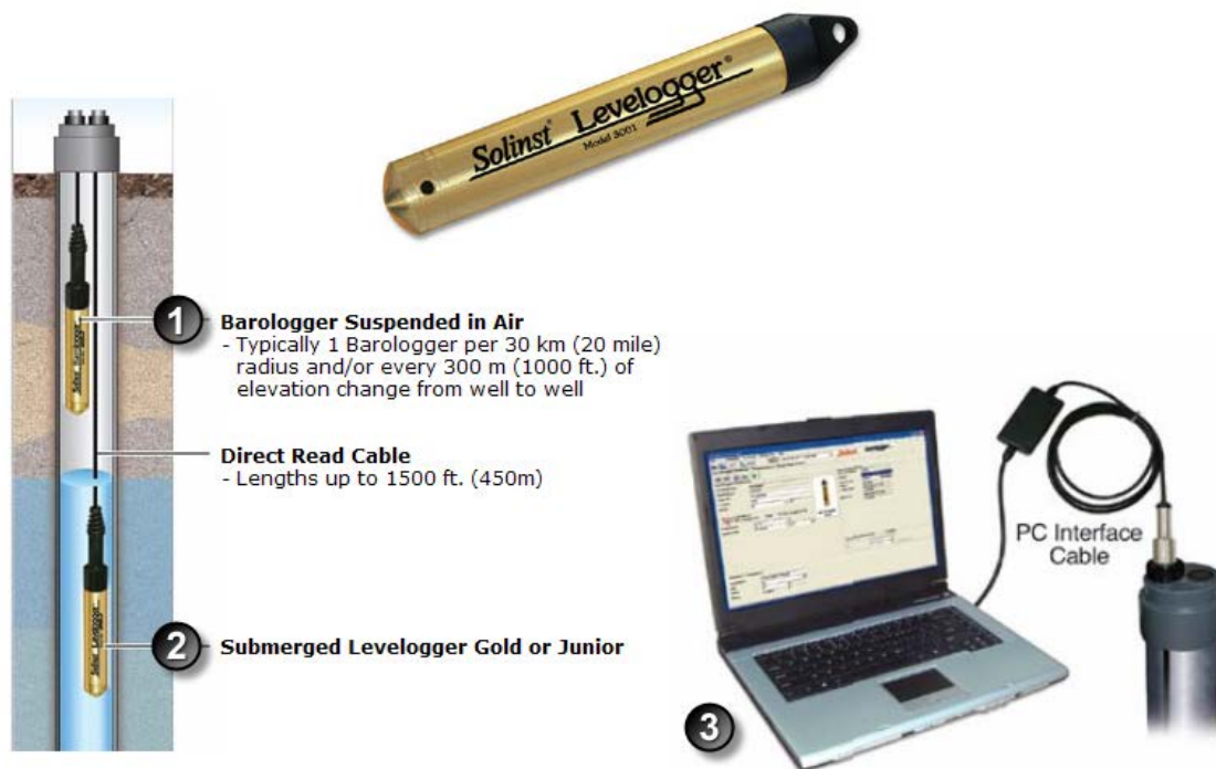
Figure SOP 15.1. Illustration of a typical deployment of the Solinst Levellogger gold unit used in SIEN pilot studies. Two loggers are required: one to measure atmospheric pressure changes (1 in figure), and a second submerged in the well (2). Data are downloaded to small personal computer or laptop (3). More information is available at: http://www.solinst.com/Prod/3001/3001-data-loggers.html
