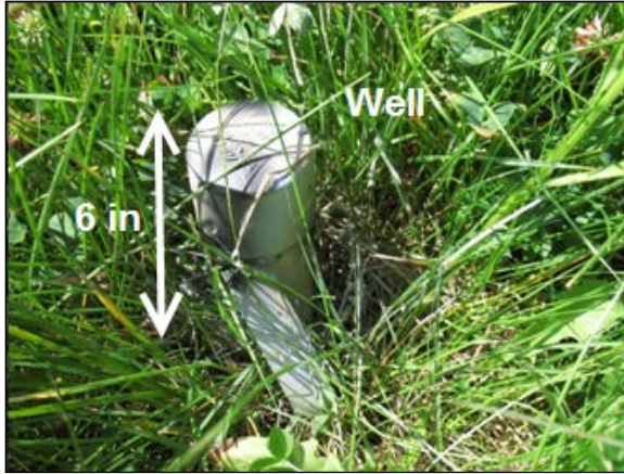
Figure SOP 8.4. Close-up photograph of well casing cut down near to the ground and painted gray to camouflage.
