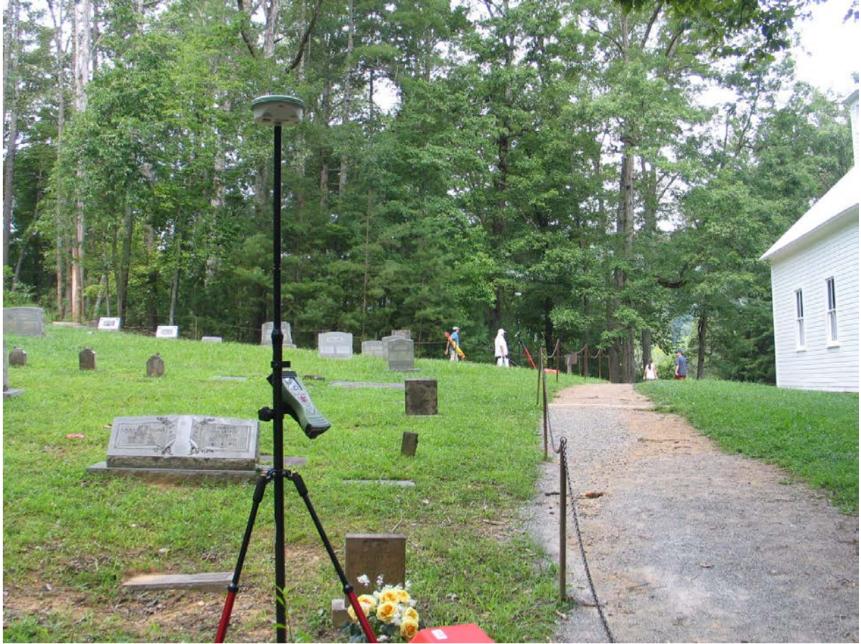
Plate 3. As an alternative to DGPS, we used an appropriate GPS Mission Plan to focus on a GPS time-window that permitted an ideal geometric dilution of precision (GDOP) during the longest sustained period. The Static GPS method used allowed us to collect ephemeris data over a minimum of four to six hours with an elevation mask of twenty degrees. This resulting high-accuracy / high-precision geographic coordinates were used to establish short baselines within each cemetery. A Total Station was then used to establish supplemental monumentation for the Robotic Total Station and C10 High Definition Laser Scanner for mapping the cemeteries.
