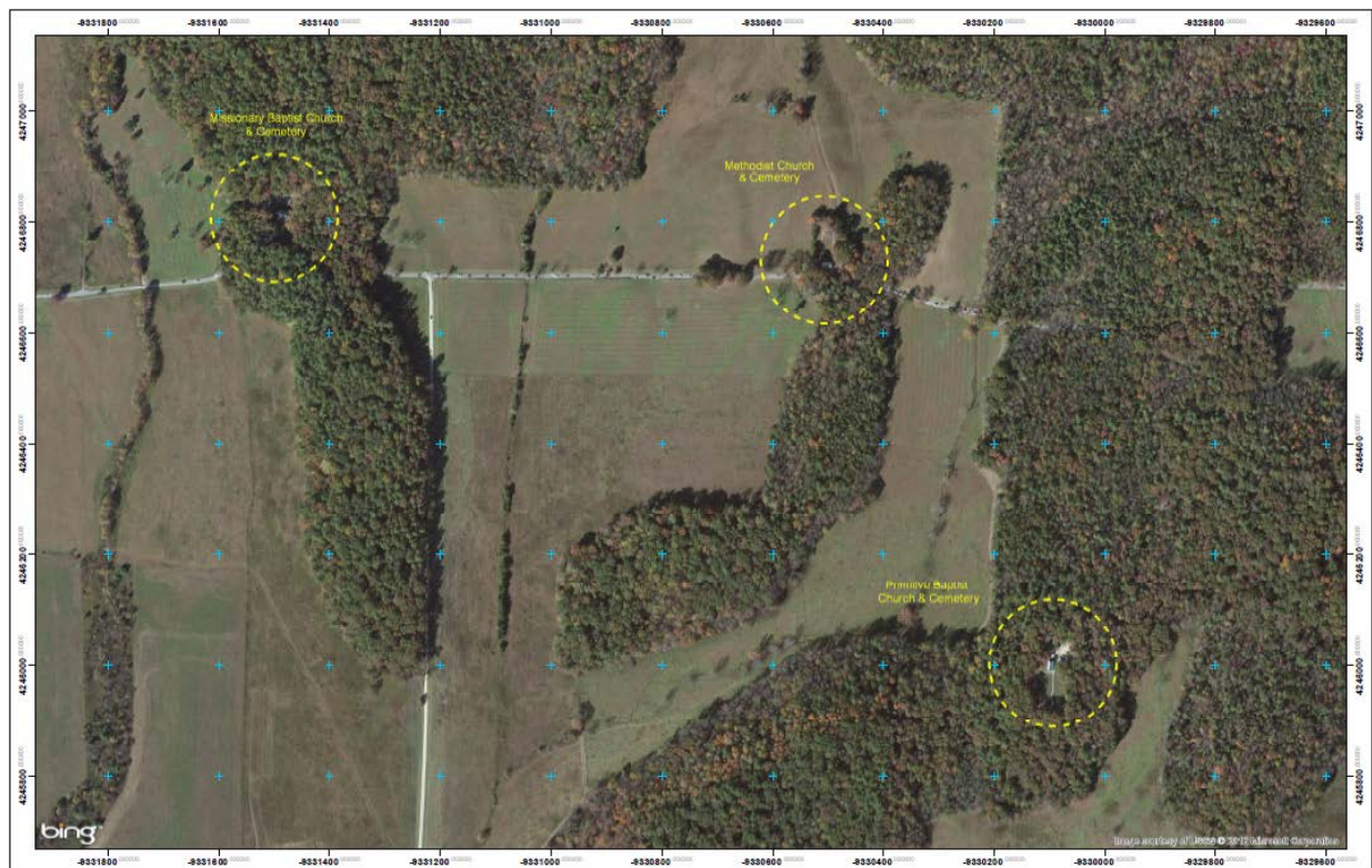
Figure 2. Heavy canopy surrounding each cemetery coupled with the Cove’s low-lying geography within the Smokey Mountains, prevents the use of differentially-corrected GPS methodologies (DGPS). Static GPS methods using long occupational times, when coupled with an appropriate GPS Mission Plan, can provide the necessary high-precision / high-accuracy coordinates needed for accurate mapping of the features within each cemetery. Missionary Baptist (left), Methodist (center), and Primitive Baptist (lower right) Cemeteries, cades Cove, TN.
