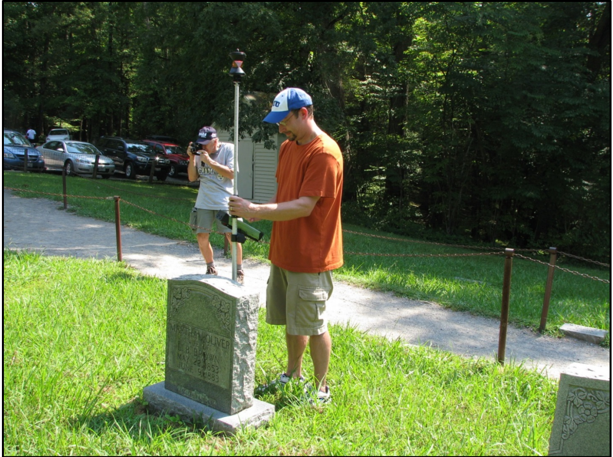
Plate 2. A robotic Total Station was used to locate individual headstones, footstones, and cornerstone monuments at each gravesite. Planimetrics (fence lines, tree lines, walking paths, and structures) were also mapped as a reference for the marker surveys for our base maps. Autonomous mapping by Dr. William Lovekamp (foreground - surveying), Dr. Vincent P. Gutowski (background – photographing), Primitive Baptist Cemetery, Cades Cove, TN.
