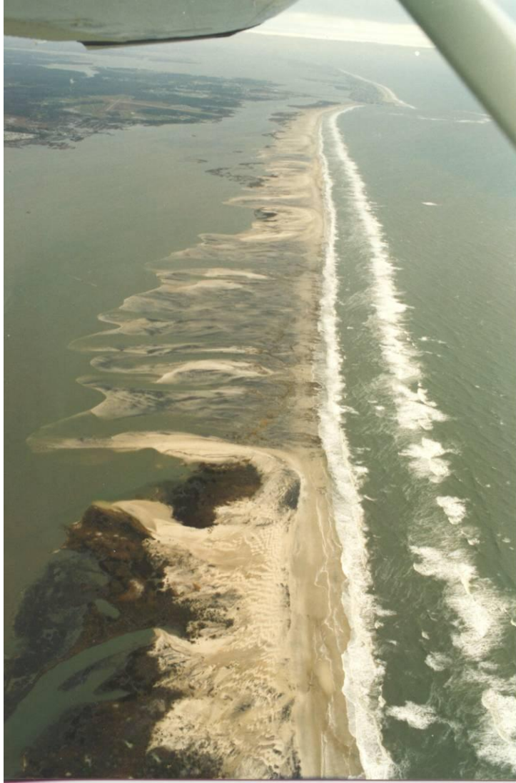
Figure 11. Two northeaster storms in 1998 caused sustained overwash that created a large overwash fan and uncovered relict backbarrier peat along the shoreline and within the island's interior. Image from Assateague Island National Seashore.
