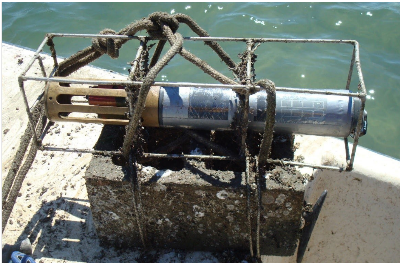
Figure 4. Photo of continuous data collection sonde and mount used at Middle Marshes (CALO2) at Cape Lookout National Seashore. Photo by John Fear.
