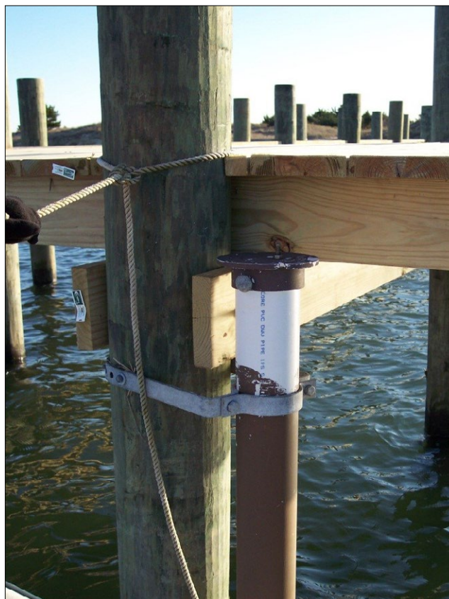
Figure 3. Photo of continuous data collection station at Shackleford Banks Dock (CALO01) at Cape Lookout National Seashore. Photo by John Fear.
