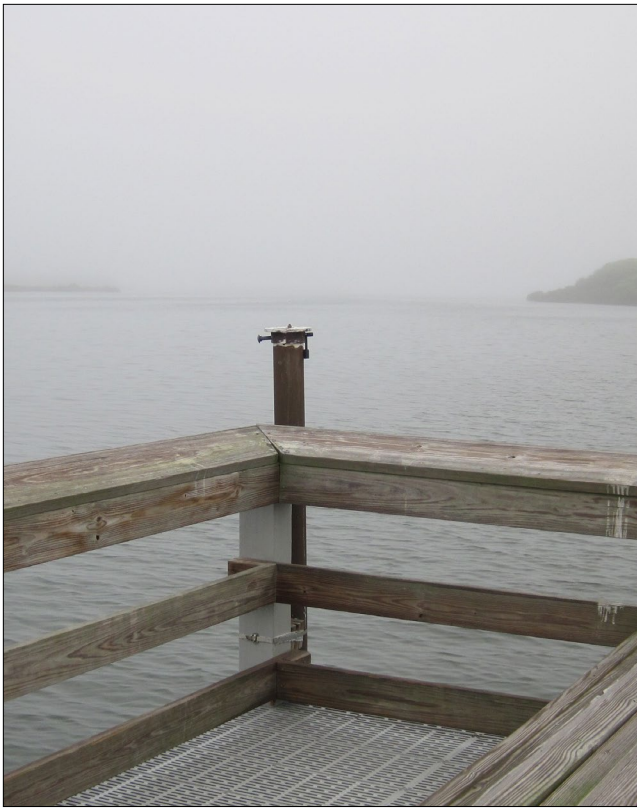
Figure 3. Continuous data collection platform used at Canaveral National Seashore. Photo shows sonde housing and locking cap. Photo by Pete Mockus, SECN staff.
