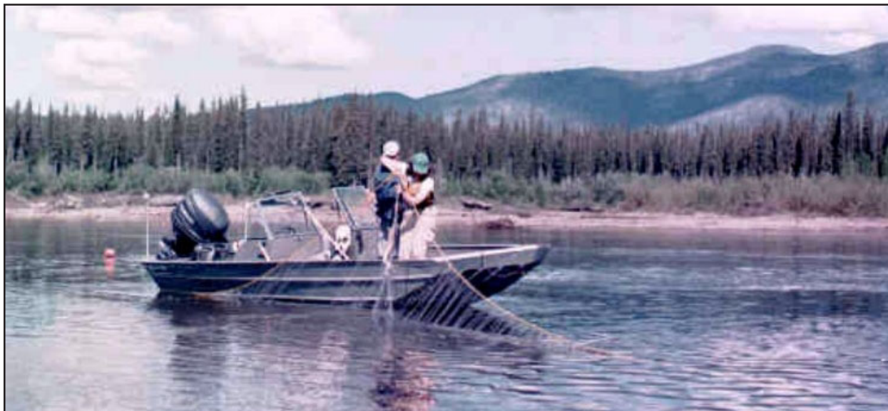
Natural resource staff check a gill net on the Kandik river during the fish contaminants study. The sampling procedure was designed to provide information on the presence, distribution and concentration of organochlorine and elemental contaminants in large river systems of the United States.
