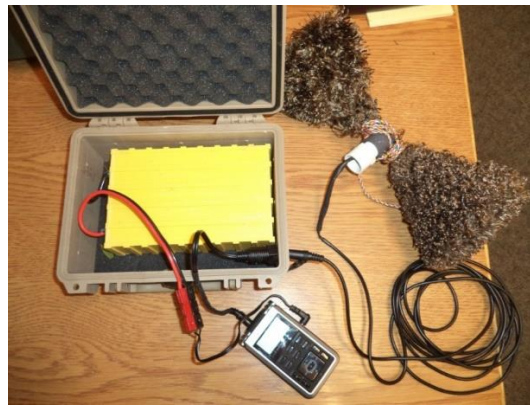
Figure 2. Components of a biological sound station
