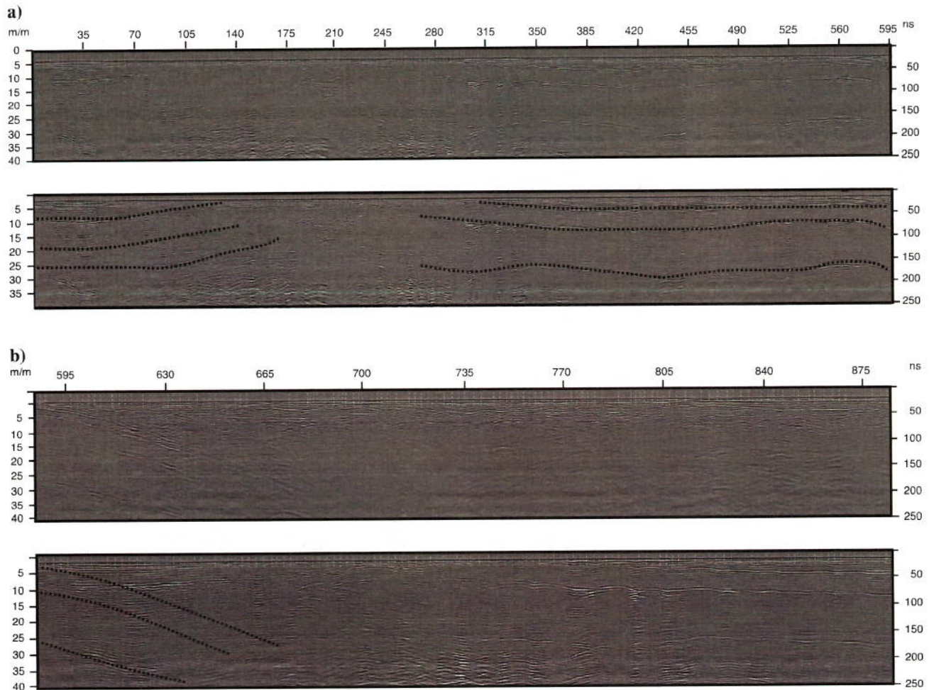
Figure 18. (a) Uninterpreted (top) and interpreted (bottom) 100-MHz GPR profile along the southern section of the road of Broken Top rift zone. Profile shows three strong amplitude interfaces (dashed lines) at depths of 5, 15, and 30 m and also a discontinuity of these interfaces for about 50 m length corresponding to faults in the area. (b) Uninterpreted (top) and interpreted (bottom) 100-MHz GPR profile along the northern section of the road of Broken Top rift zone. Three strong interfaces dip toward the rift area, where there is no clear definition of interfaces.
