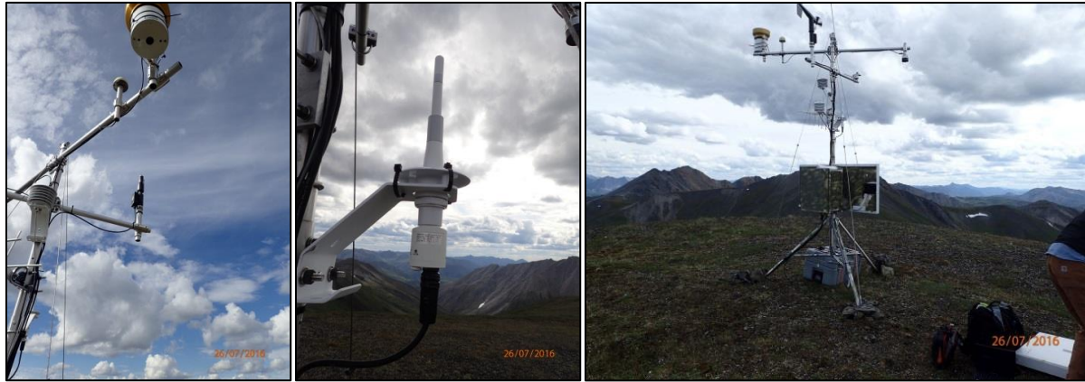
Figure 18. Imelyak climate station, July 26, 2016. Upon arrival, the WS-WD sensor (left) and 14-plate radiation shield (middle) were missing. The WS-WD sensor was replaced on 7/26/2016 (right). The radiation shield was replaced on 8/12/2016.
