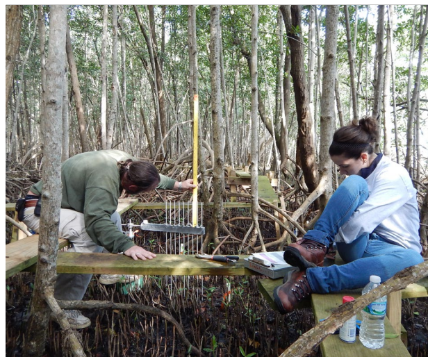
Figure 1. Kevin Whelan (Ecologist, National Park Service) measures soil surface elevation using the Soil Elevation Table (SET). The SET is a sampling device that is attached to a permanent benchmark. The height of the pins transcribes the elevation of the soil and standardizes it to a fixed reference point (the metal arm). Repeated measurements over time monitor the rate of soil elevation change.
