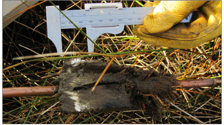
Calipers measuring accretion at a salt marsh site in Cape Hatteras National Seashore.
