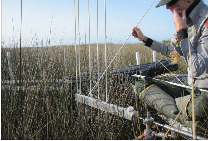
A coastal ecologist measures saltmarsh elevation using a Rod-Surface Elevation Table technique at Cape Hatteras National Seashore.
