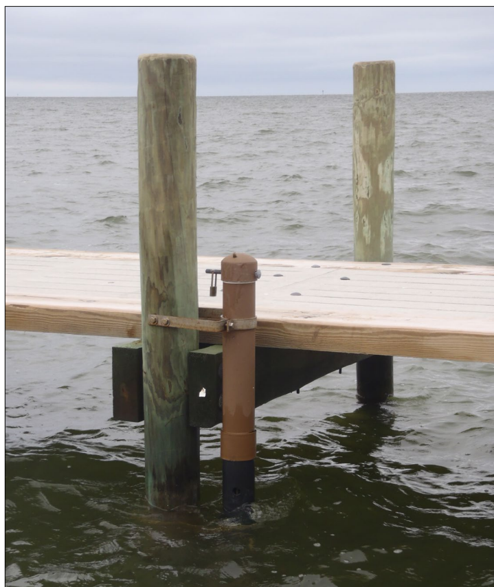
A data sonde is secured inside a guard and mounted to the dock at Cape Hatteras National Seashore.
