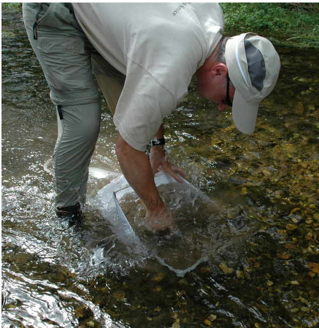
Collecting invertebrates with a Surber sampler. (NPS)
