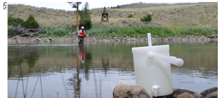
River sampling at the Lamar River using a churn splitter to produce a representative sample of river conditions. NPS PHOTO.
