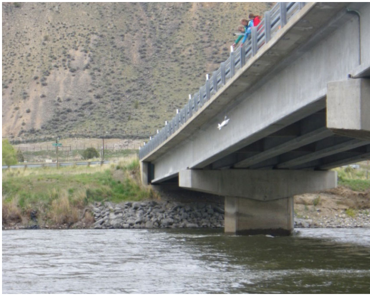
During high flow conditions, river sampling is accomplished by lowering a suspension sampler and collection bottle with a reel and bridge board (Yellowstone River at Corwin Springs, MT).
