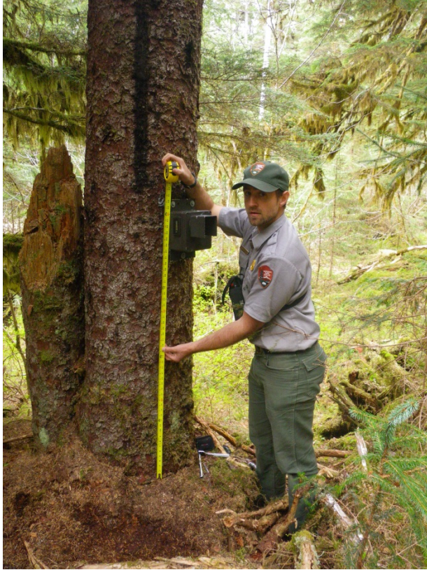
Figure 4. Ivan Technologies infrared trail event counter receiver installation.
