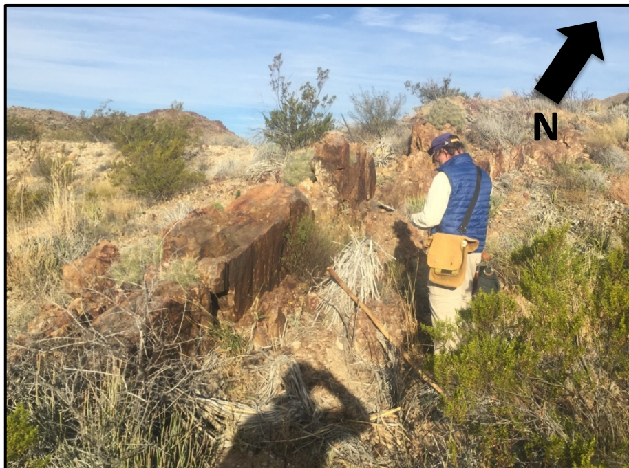
Figure 4.36 – The fault plane of major normal fault MN-4 (S196) which is associated with large outcrops of red-stained vertical “fins”.
