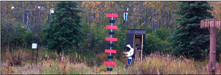
Figure 4. Kantishna SNOTEL station. The gage on the right measures precipitation year-round. The red and black totem is an aerial marker for snow surveys. Sensors on the tower on the left measure snow depth, temperature, and rainfall.
