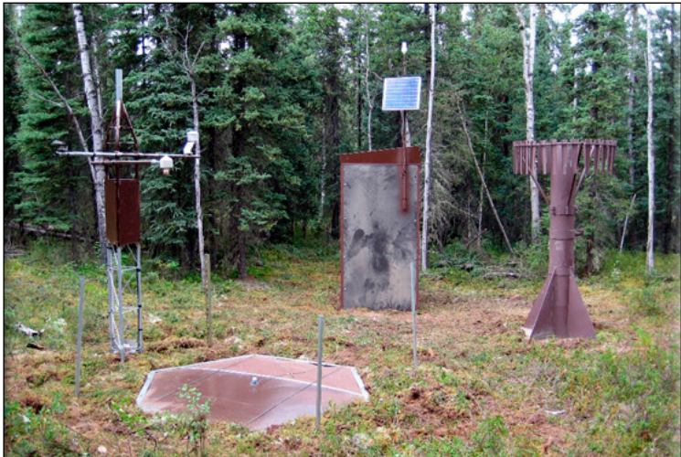
Figure 4. American Creek SNOTEL station. The gage on the right measures precipitation year-round. Sensors on the tower on the left measure snow depth, temperature, and rainfall.
