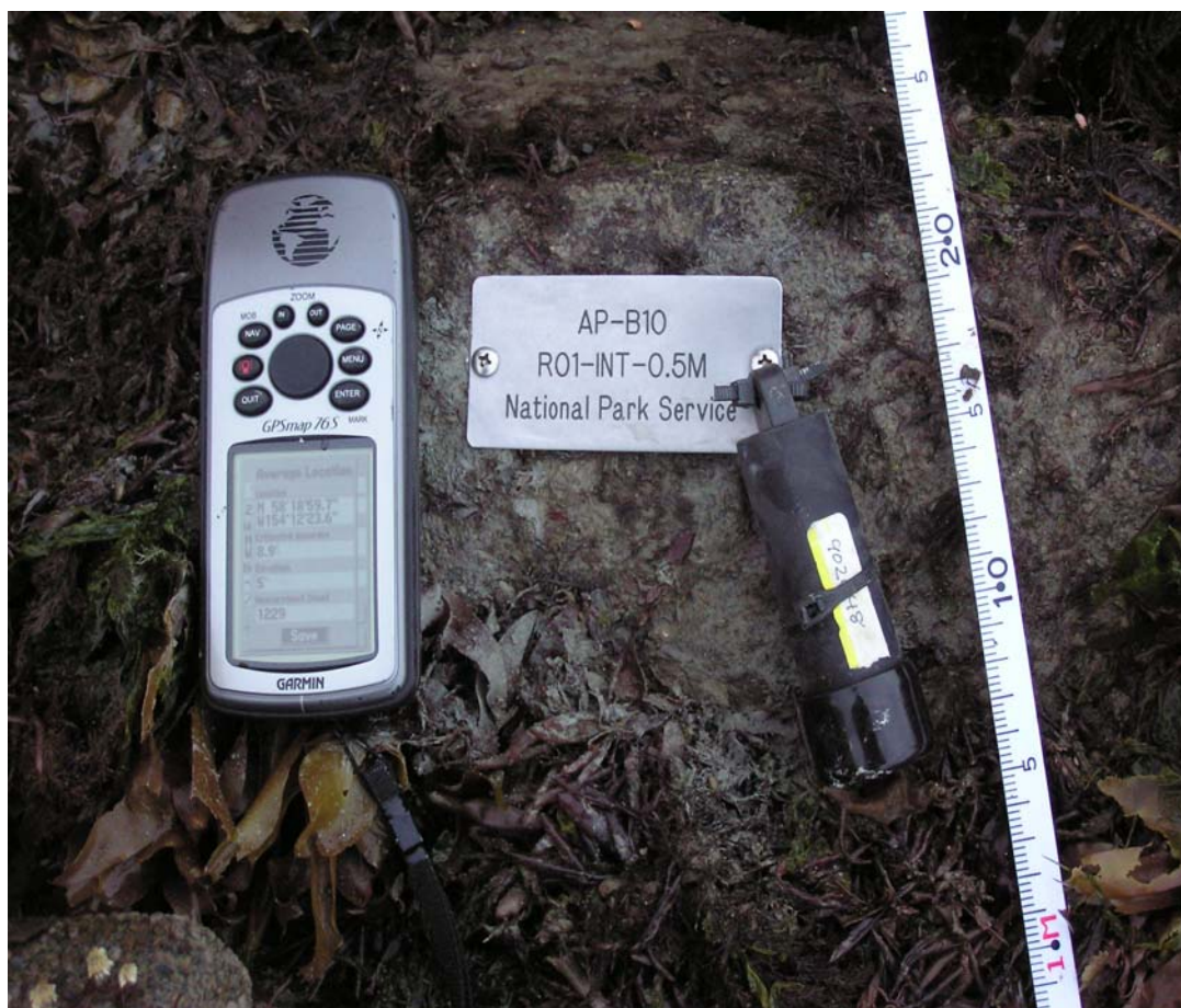
Figure 2.2. Stainless steel marker bolted to substrate at zero end and +0.5 m tidal elevation of 100 m transect at site AP B10 RI1, with HOBO temperature recorder and GPS used to obtain coordinates.
