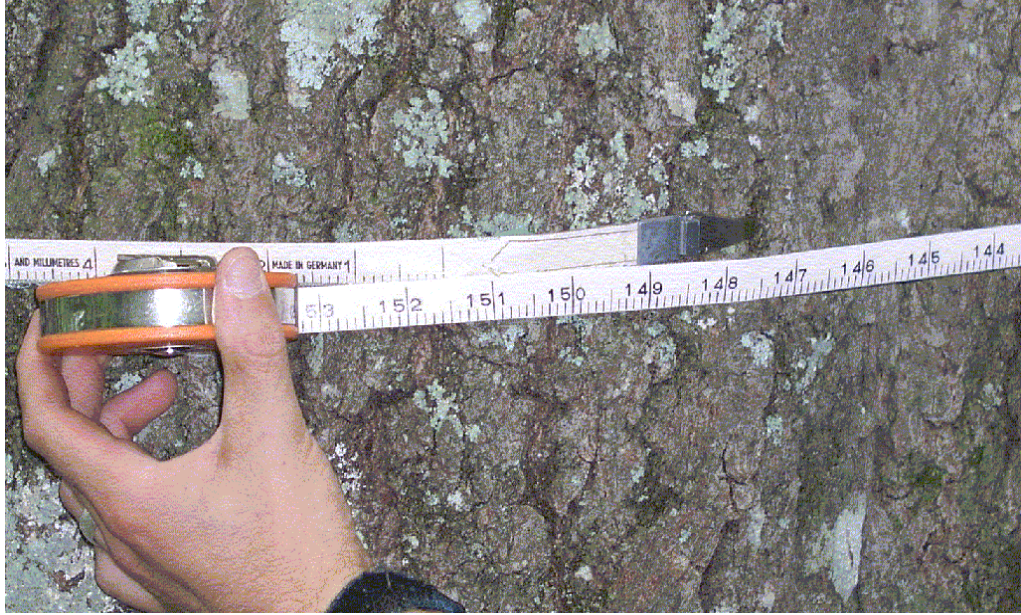
Figure 1. The proper method for securing a DBH tape.
