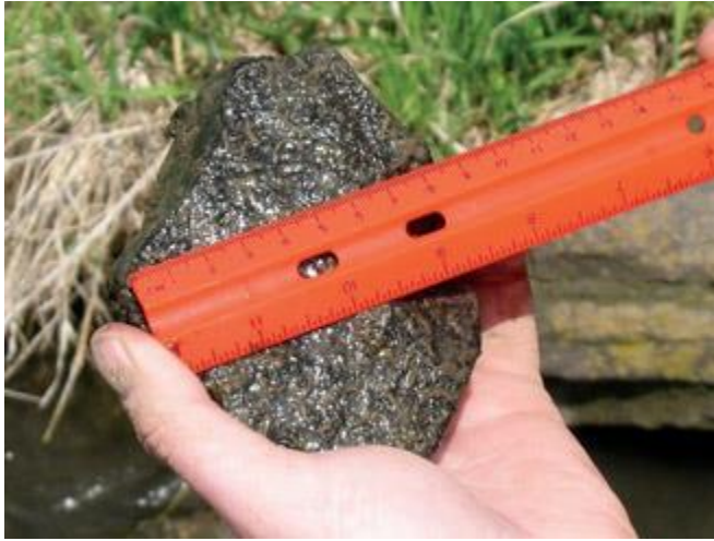
Fig. 1. Measuring the intermediate axis. Note its position relative to the longest axis (the vertical axis in this image) and the shortest axis (pebble depth in this image).
