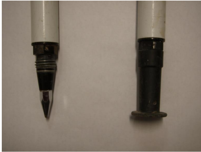
Figure 2. Options for the bottom of prism poles. The point on the left is used for control points, top of headpins, and well shots while the flat foot on the right is used for all other shots. Leveling rods only have a flat foot.
