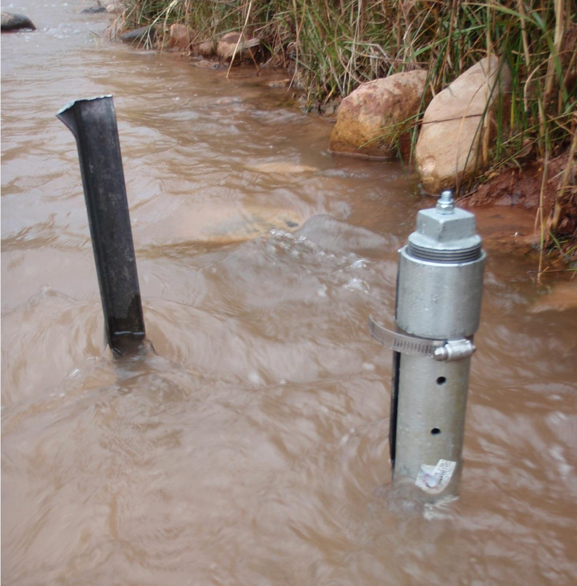
Figure 10. Angle iron installation in Fremont River, CARE.
