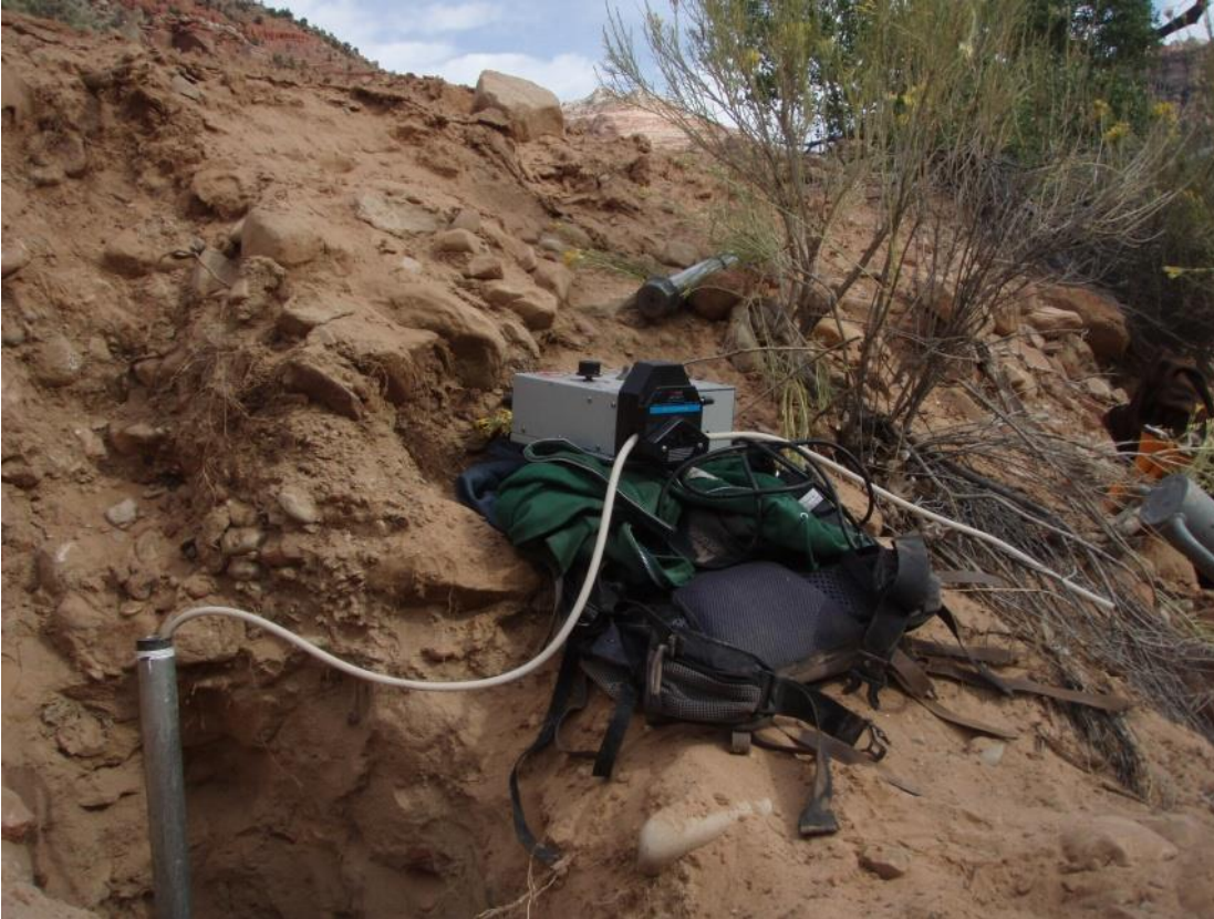
Figure 6. Pumping a well with a peristaltic pump at the East Fork of the Virgin River, Zion National Park.
