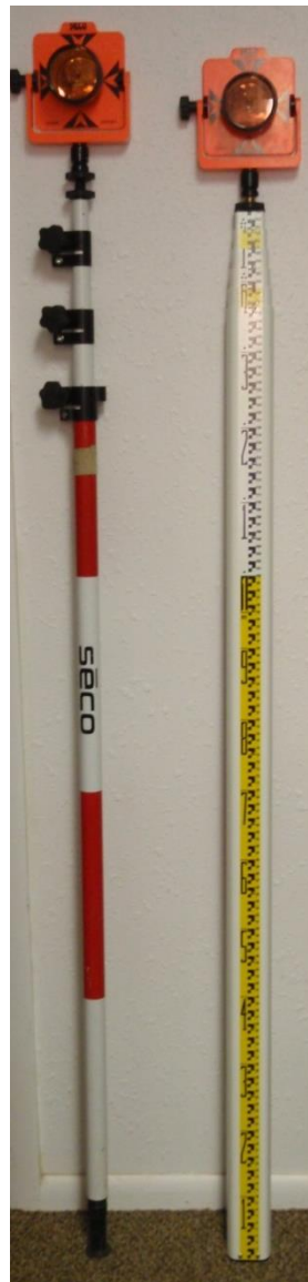
Figure 1. Photo of a prism pole on the left and a leveling rod on the right.
