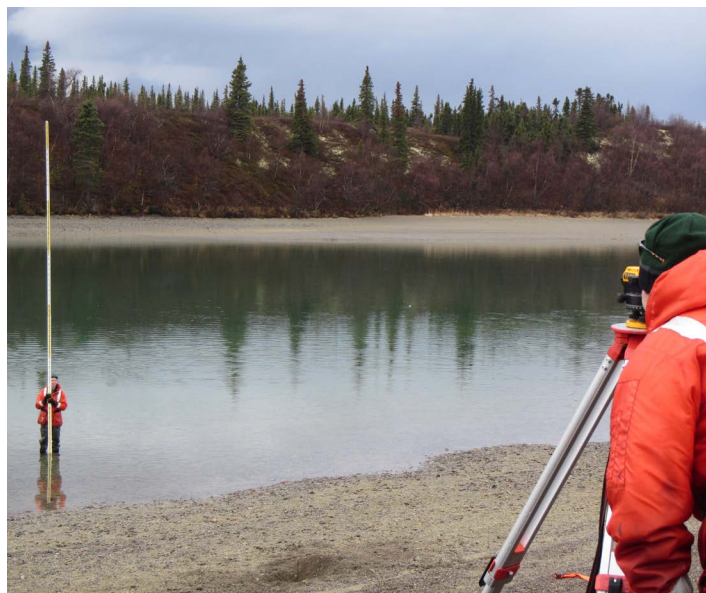
Using a transit level (right) and stadia rod (left) to survey level logger elevation at the outlet of Lake Clark in Lake Clark National Park and Preserve.
