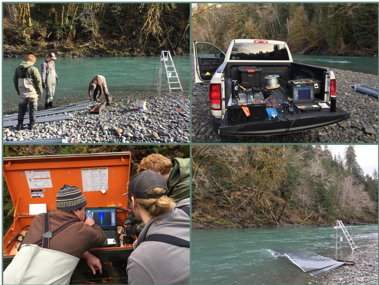
Figure 3. The field team sets up the sonar unit at our field site in late January 2017. An aluminum ladder is used to position the sonar in the river. A finger weir is used to divert shore-oriented fish in front of the ladder and sonar unit. Data collected by the sonar are stored in computer files for analysis.
