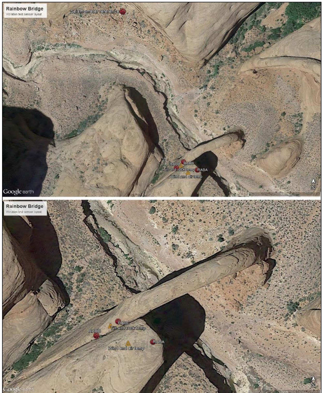
Figure 1. Overview of sensor locations on and around Rainbow Bridge. Reference seismometer is RABD. RABB and RABC are 12.5 m apart on the bridge; RABA is on the adjoining knoll. (Google Earth).
