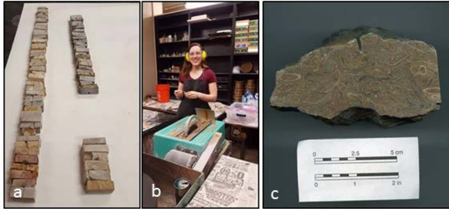
Figure 5. a. At the UTSA Geology Rock lab, 81 billets prepared for thin sections; b. cutting Santa Elena Canyon samples with rock saw prior to polishing; c. polished sample ready for describing.
