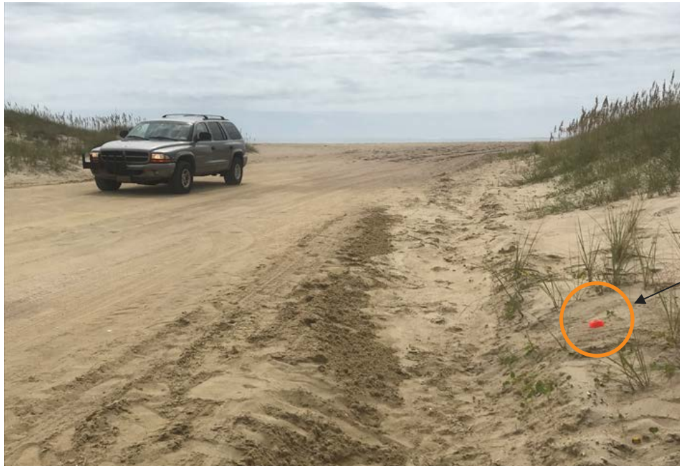
FIGURE 8. RAMP 44 MAGNETIC VEHICLE COUNTER DEPLOYMENT SET UP
